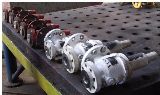
Overhaul of PV valves
