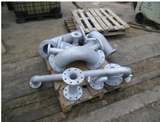
Blasted and galvanized pipe
