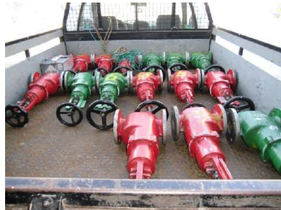
Completed PV valves
