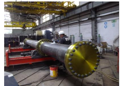
Spools assembled for pressure testing
