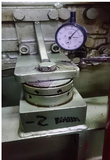
Alignment: 2mm in axis 3
