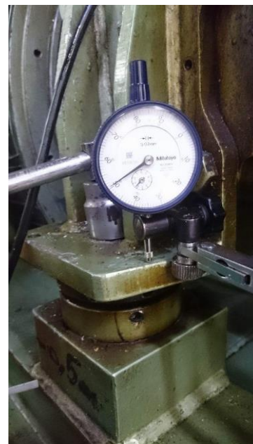
Alignment: 0,5mm in axis 2
