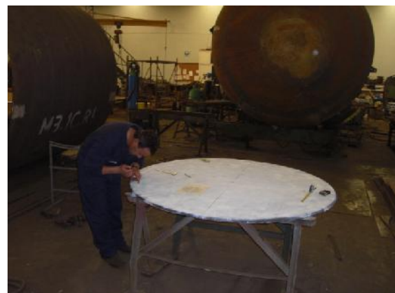
Marking of tube plate in workshop
