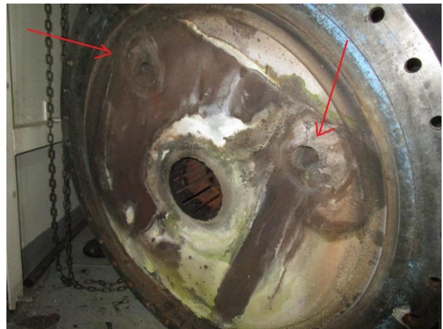
Visible cracks on the pilot burner hole and peep hole, view from bottom plate of cooling chamber
