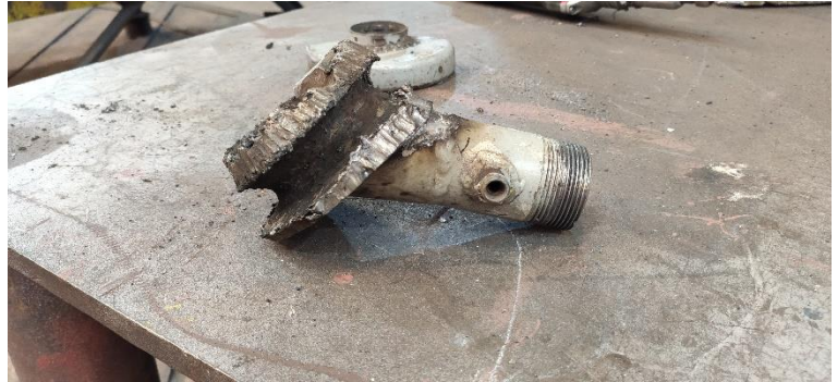
Removal of the pilot and peep pipes, including the steel damaged areas.
