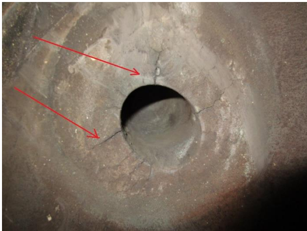
Visible cracks on the pilot burner hole and peep hole, view from bottom plate of cooling chamber
