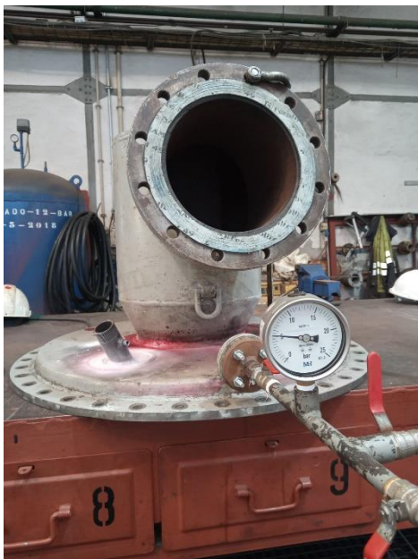
Finally, the hydraulic pressure test. No leaks were detected.
