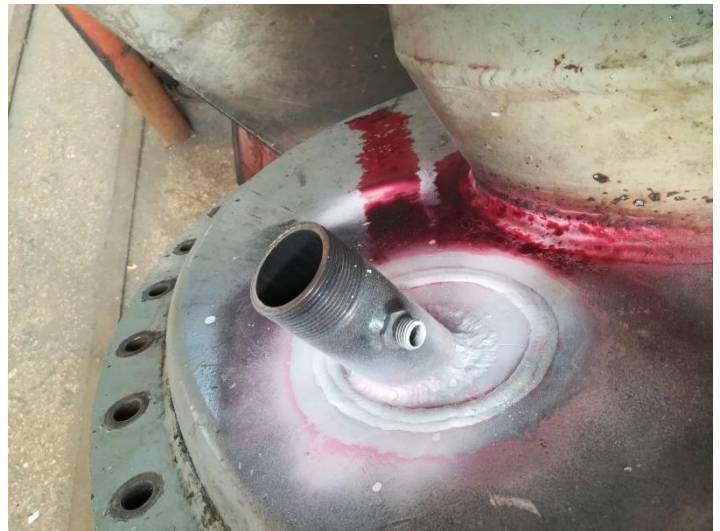
After welding all welds seams were inspected with dye penetrant. No defects were found.
