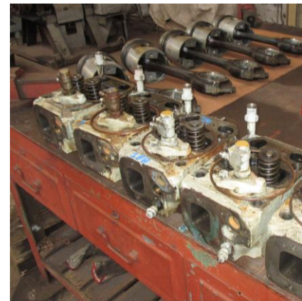
Main engine overhaul
