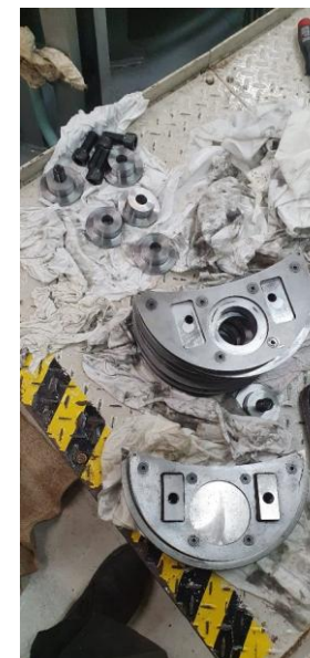
Rudder steering gear opened and preparation for its cleanliness.
