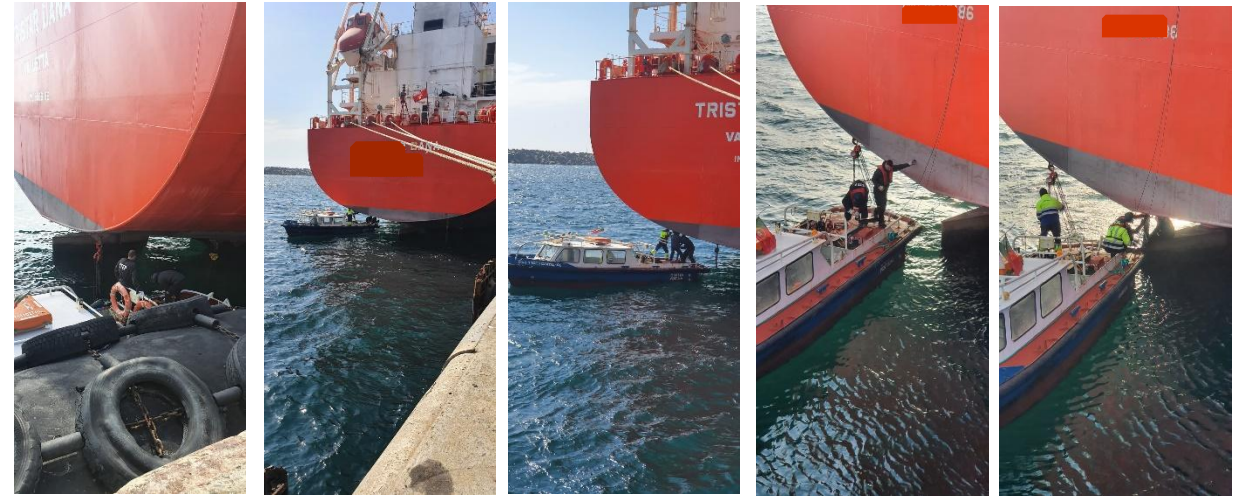
Floating jobs with barge for the rudder preparation.
