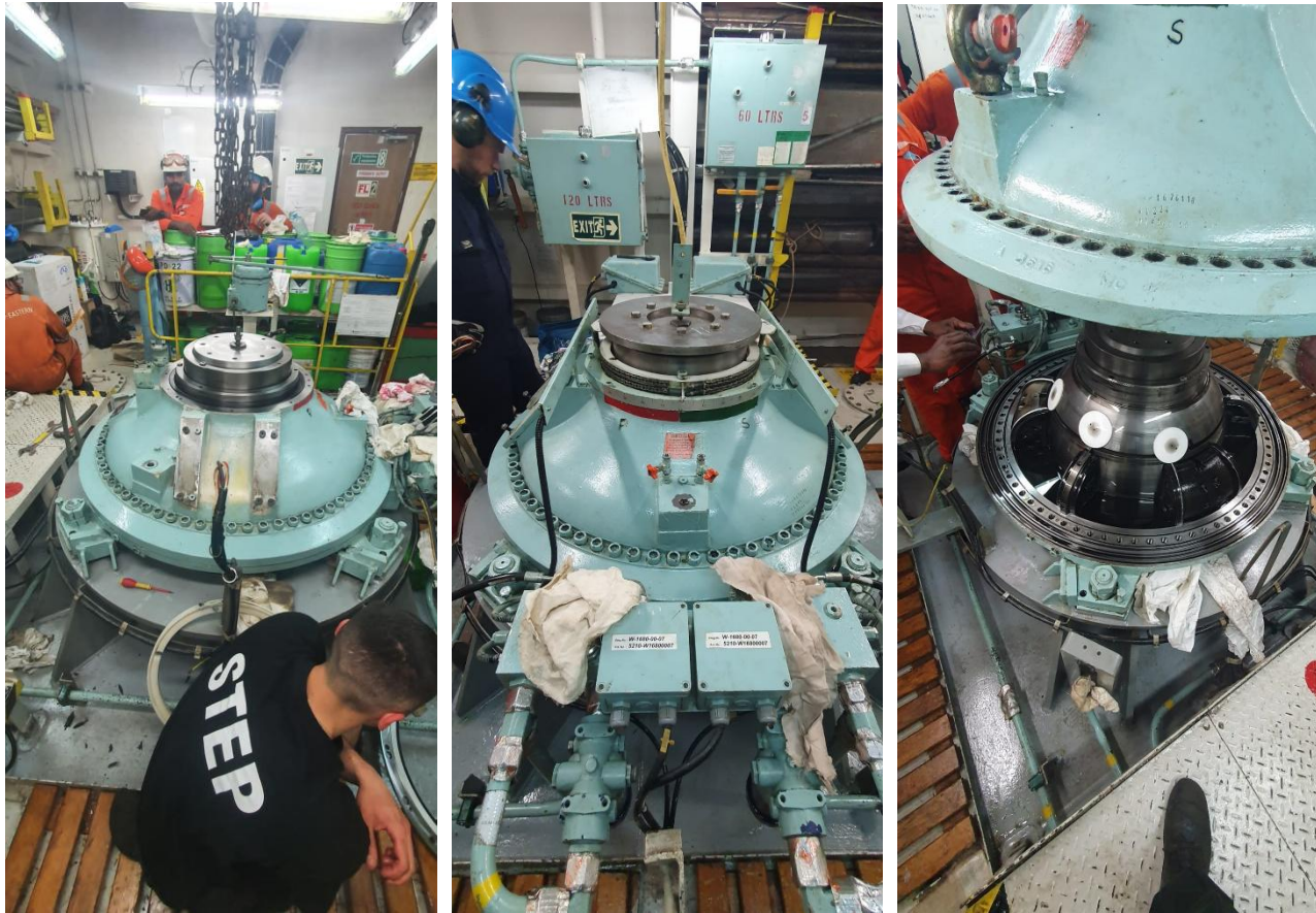
Rudder steering gear opened and preparation for its cleanliness.
