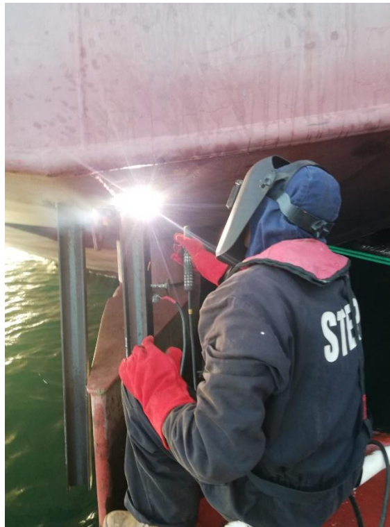
Rudder immobilization by mean of chain blocks and bar welding.
